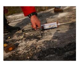
using water (pressure wash), brushed and washed until all the limestone dust had been removed, the holes were then dried using absorbent cloth. The anchors were secured in the substrate using R-KER Epoxy Acrylate Styrene free resin. This is manufactured by RAWL Fixings. The anchors were left unloaded for 3 days until test to failure on 05<sup>th</sup> October 2011. On 05<sup>th</sup> October 2011 twelve anchors were tested to destruction.
